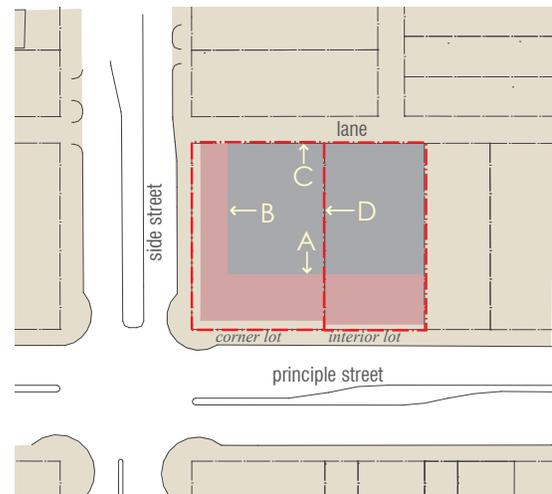
Vehicular access permitted only from rear lane. At-grade parking (enclosed and unenclosed) should be placed in the shaded area shown.
